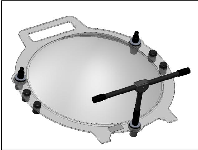
Step 2 - Install right-hand and left-hand handles and snap onto the horizontal cross bar
